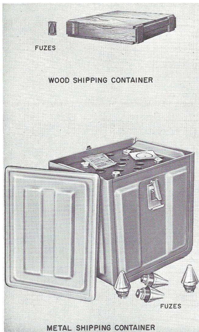
Figure 3-20. Typical Fuze Shipping Containers
