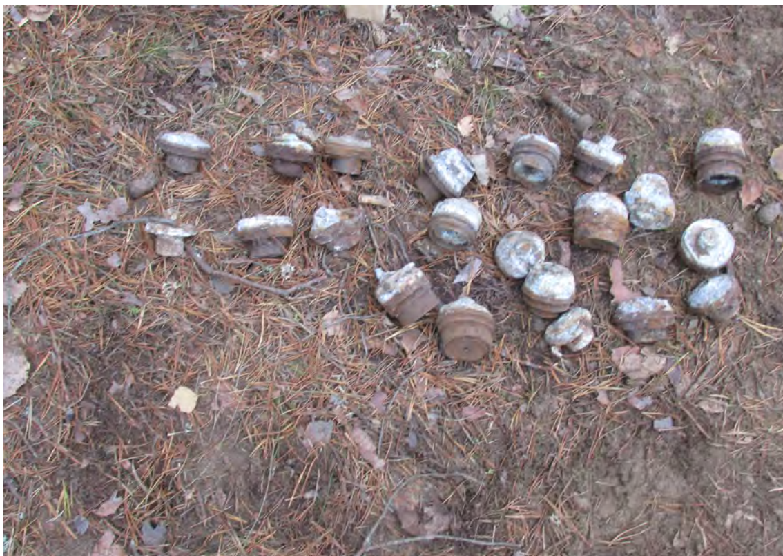
Image 114. Effects of ageing visible on pyrotechnic time fuzes (source: GICHD ©)
