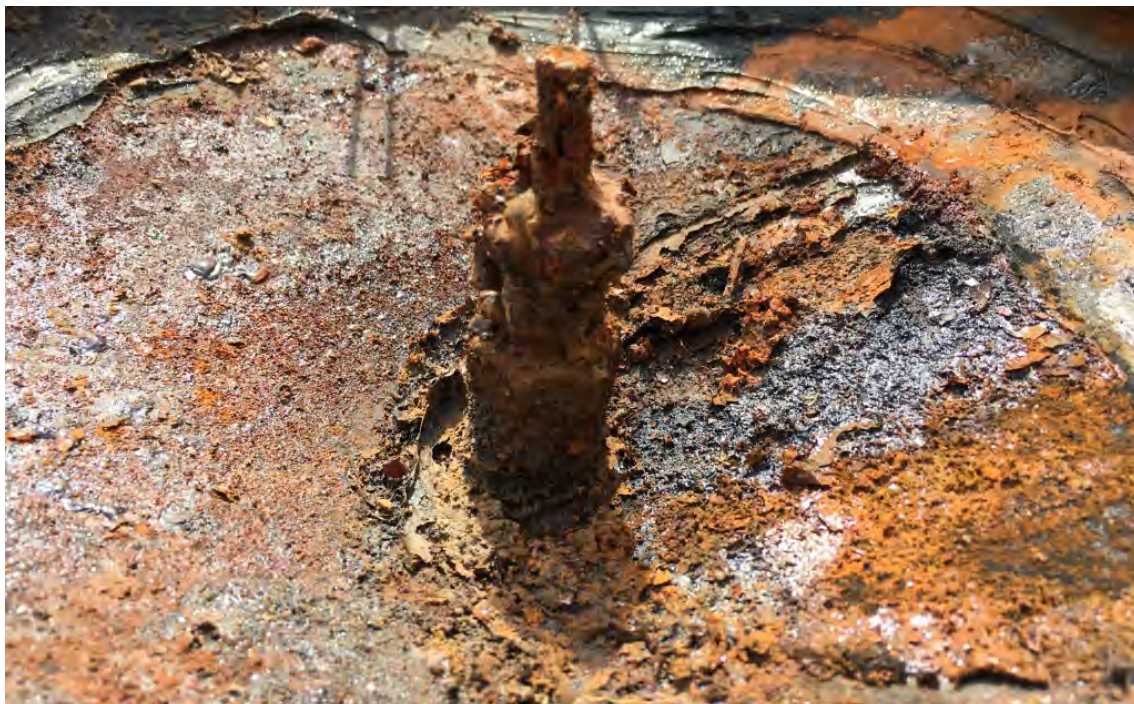
Image 116. Cocked striker of a VS-500 corroded by ageing (source: FSD ©)
