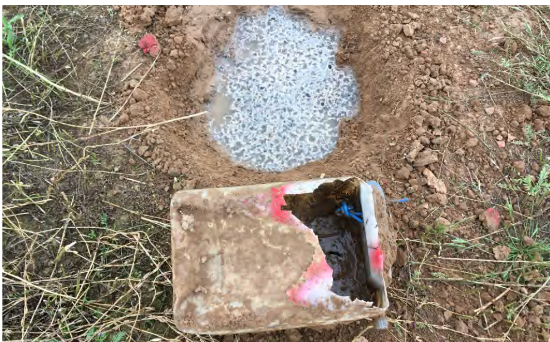
Image 117. Effects of ageing: aluminium powder after separation from ammonium nitrate (source: FSD ©)
