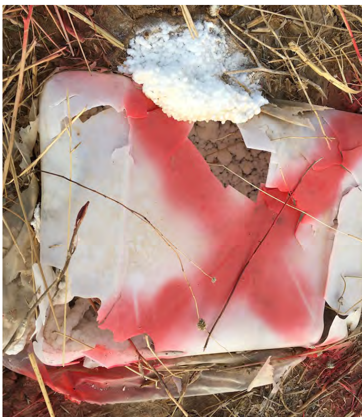
Image 119. Effects of ageing: recrystallised ammonium nitrate (source: FSD ©)
