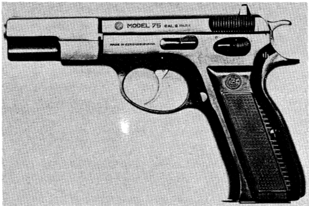
Figure 32.2. The Czechoslovak 9-mm Vz75 pistol.
