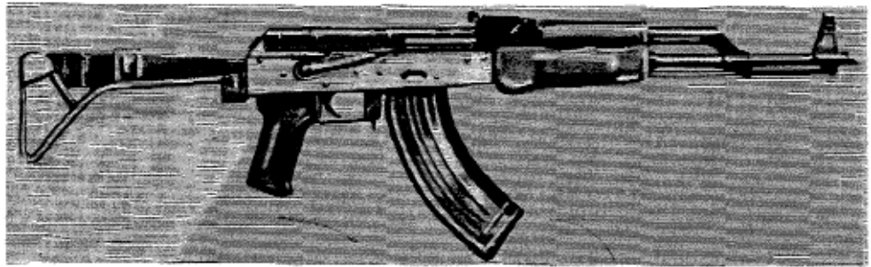
Figure 83.3. East German MPiKMS72 assault rifle.
