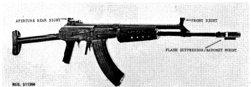
Figure 65. Finnish M60 assault rifle.
