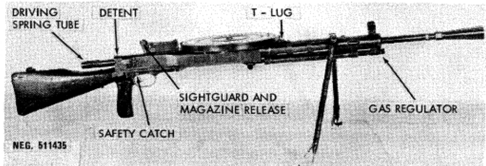
Figure 136. DPM light machinegun.
