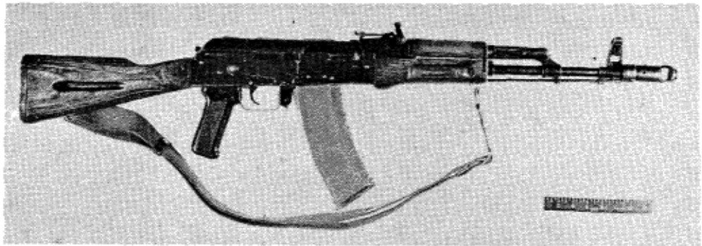
★ Figure 90.2. The Soviet 5.45-mm AK-74 assault rifle.
