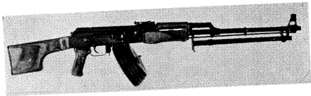
Figure 128. RPK with 75-round drum magazine.
