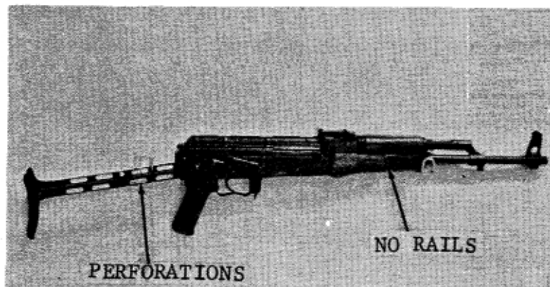
Figure 87. North Korean Type 68 assault rifle (folding stock).
