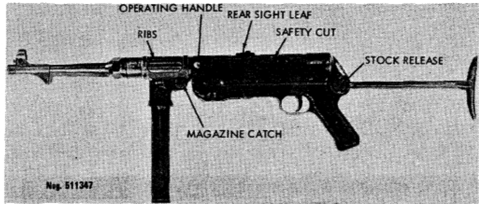
Figure 48. World War II German Model 1938 submachinegun (MP 38).
