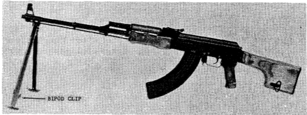
Figure 126. Soviet RPK squad light machinegun w/40-round box/magazine.
