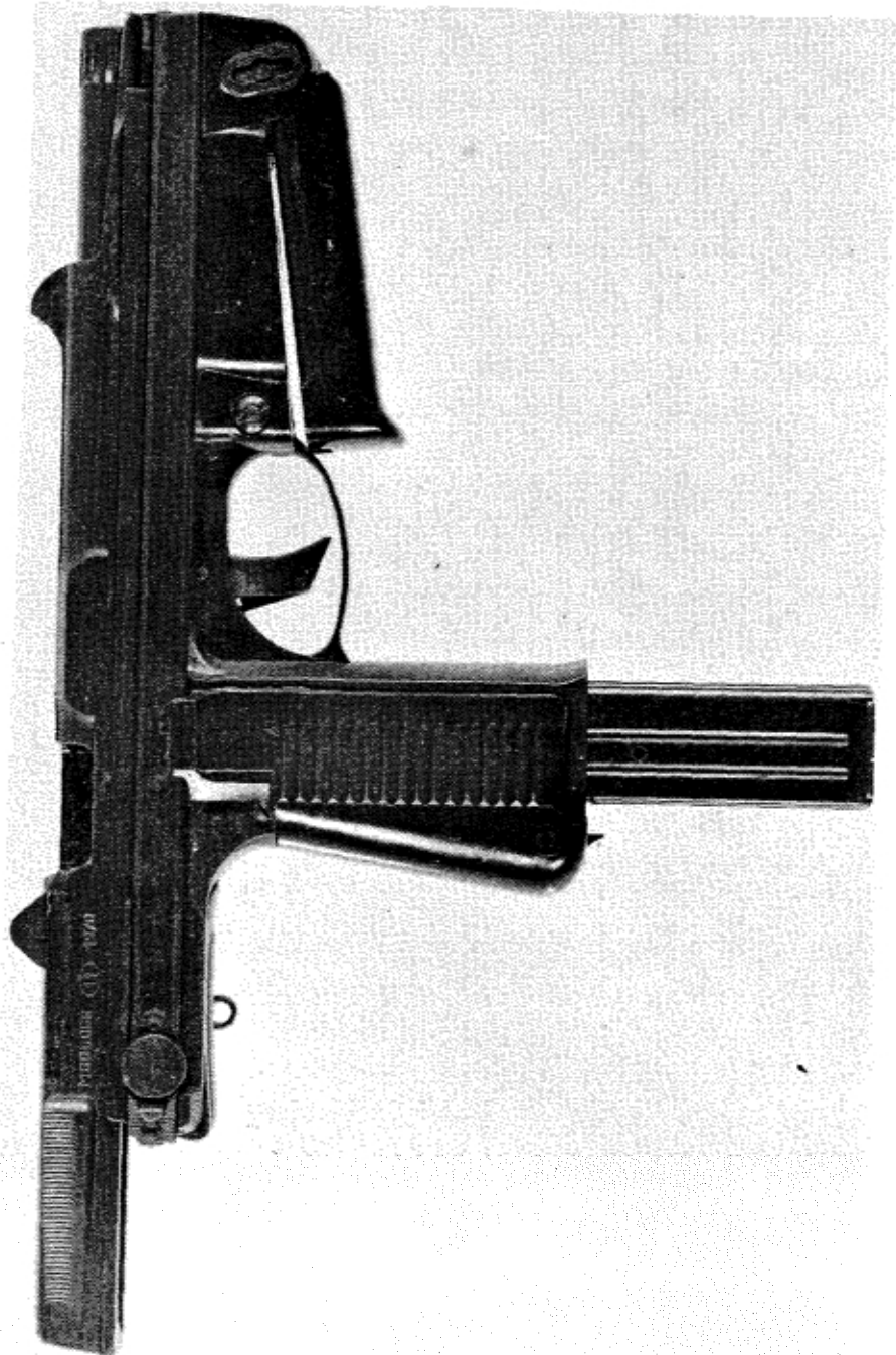
Figure 28.1. Wz63 ready to fire (as a pistol).
