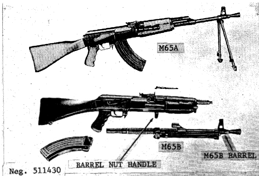
Figure 131. Yugoslav M65A and M65B light machineguns.
