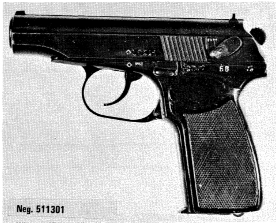
Figure 2. East German Pistole M.
