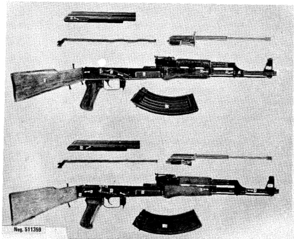
Figure 60. Differences between late (top) and early model Soviet AK-47's.
