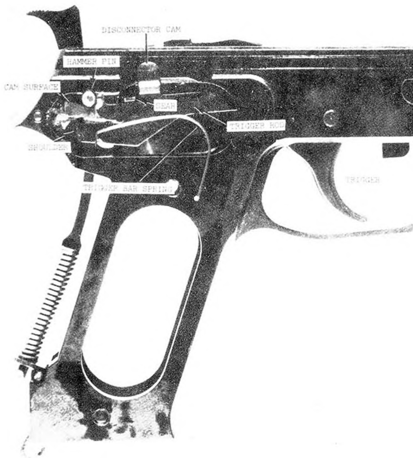
Figure 28.1.5. Model 75 trigger mechanism, at rest.
