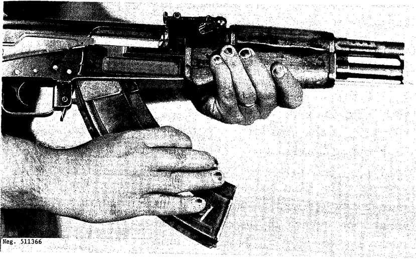
Figure 67. Inserting magazine into the AK-47.
