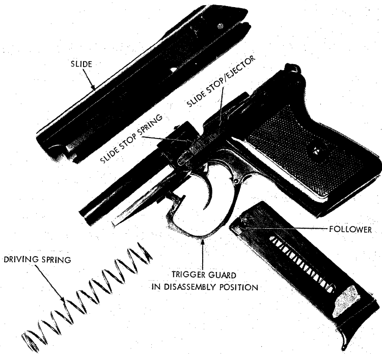
Figure 16. P-64 pistol disassembled.
