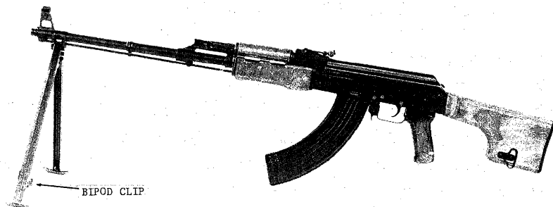
Figure 126. Soviet RPK squad light machinegun w/40-round box/magazine.
