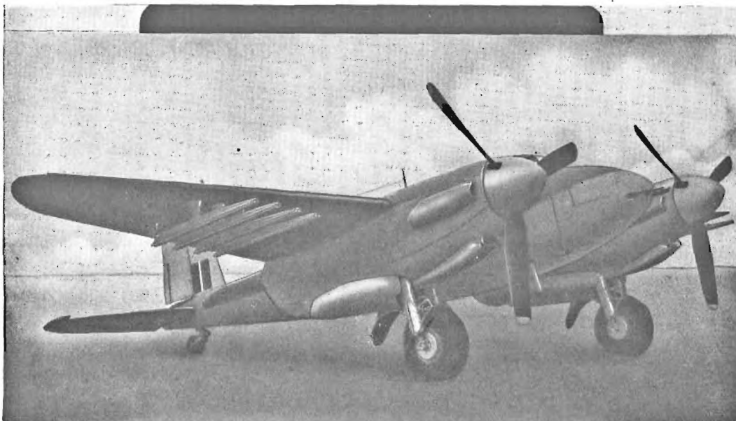
FIG. 1. The Mk.IB R.P. installation in the Mosquito aircraft
